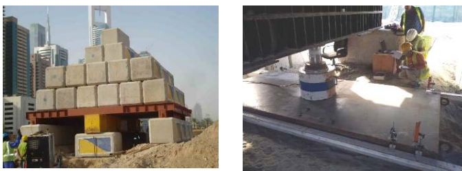
Fig. 12. Set up of zone load test
